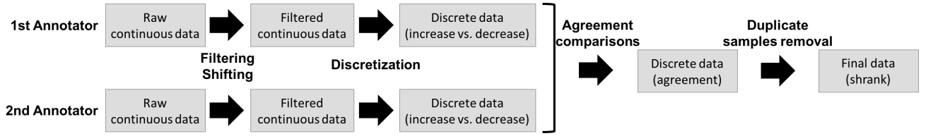
Figure 4: Pipeline of pre-processing of continuous annotations. Data are first processed separately, then last steps are performed only on time windows where the two annotators agreed.
